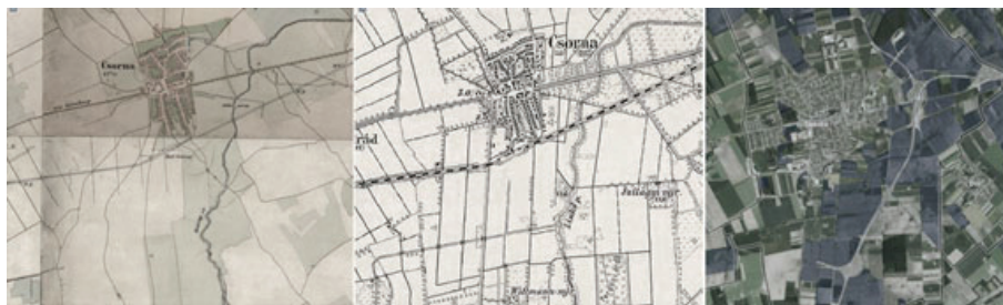
Figure 4. Land use in the middle of 19 th century in the micro region of Csorna (II. Military survey, 1845-1846); at the end of the 19 th century (III. Military survey 1872-1884); present state with frequent occurrence of excess waters
